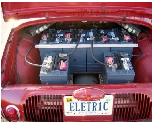
Rear-mounted batteries of a 1960 model
